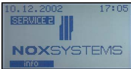
Display of maintenance level
